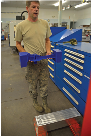
At the feet of Tech. Sgt. Richard Towlson is a 100-lb. aluminum piece just like the one used in making the C-5 part. In his hands he holds a test copy in machinable wax that was created in the milling machine.
