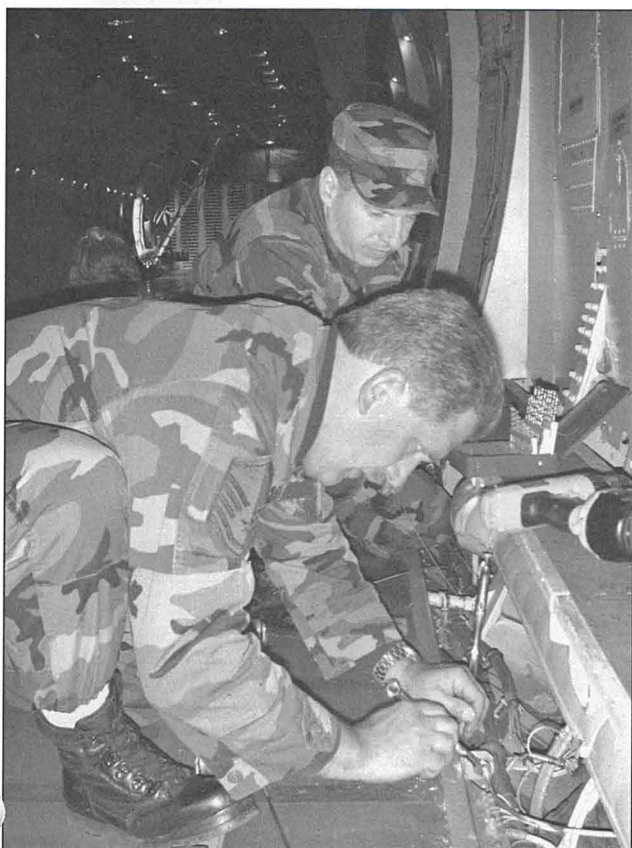
WIRED — MSgt. Joe* assists of SrA. Benjamin* replaces a detent cable on one of the many pallet locks in the C-5 cargo bay.
