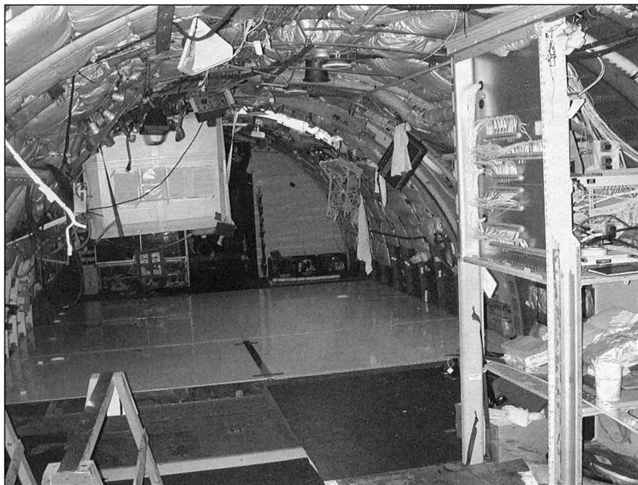
FLOOR SHOW — The C-5 flight deck is stripped to replace floor support beams and panels and other inspections and repairs.
