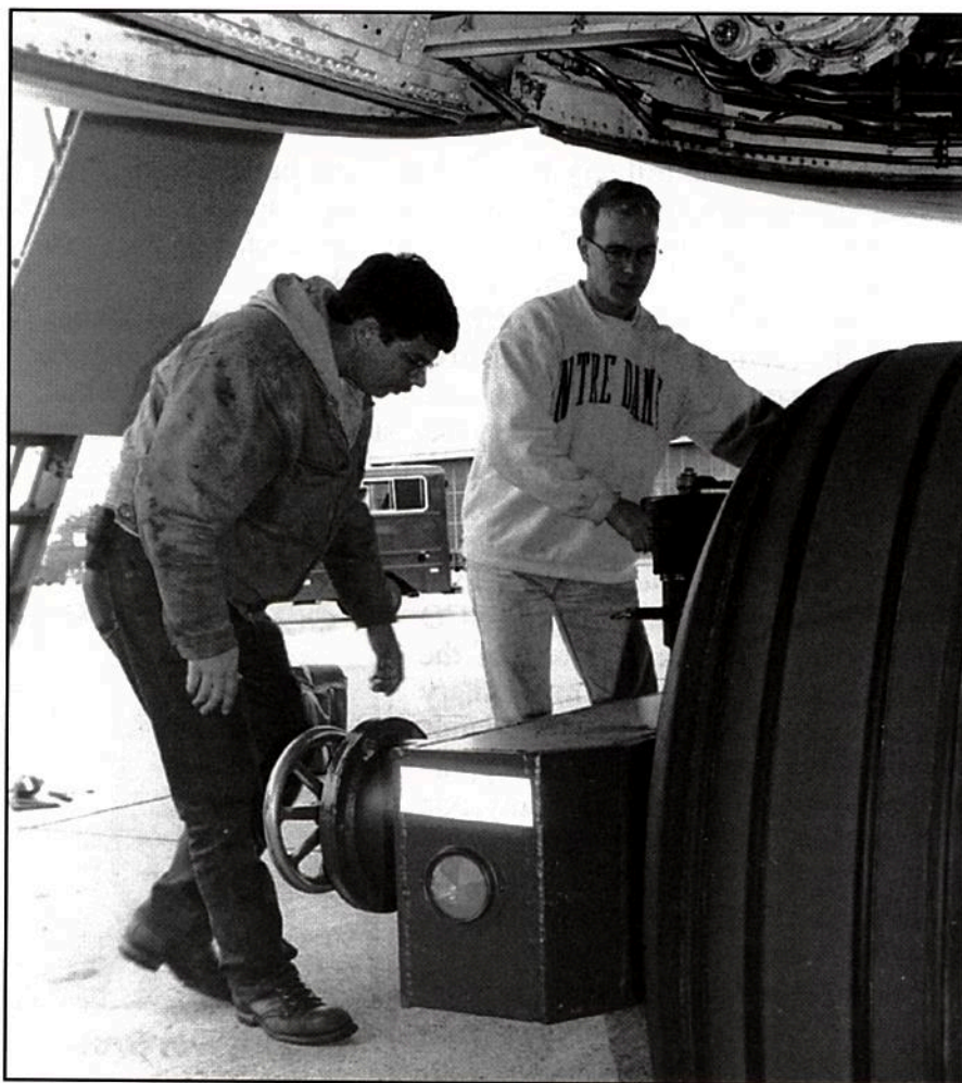
TOW JOB -- Moving a 180-ton airplane is no small task. Personnel from the 439th Aircraft Generation Squadron attach a tow vehicle to the C-5 landing gear to move the Galaxy. The ramp was cleared while lines were repainted on the flightline.
