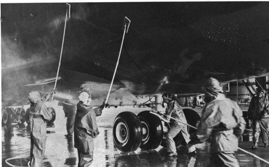
WASH AND FLY --Westover's AGS personnel scrub all 42,540 square feet of the C-5 with new wash rack equipment in the pull through hangar.
