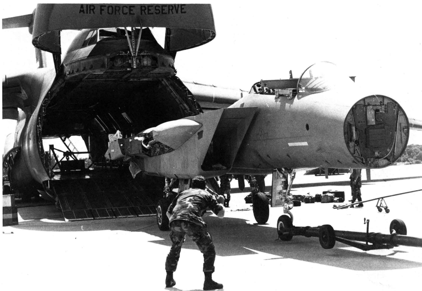
IN PLANE VIEW — 58th aerial porters guide the F-15 fuselage onto the Galaxy. The crew used a 40k-loader
