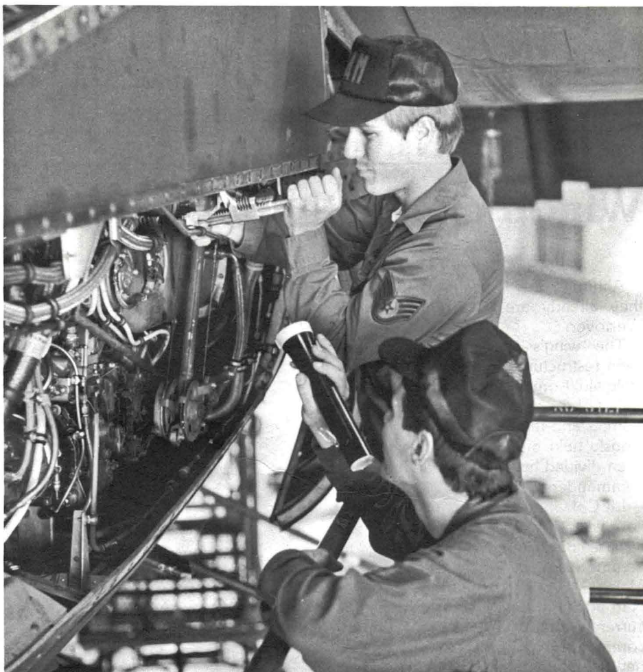
SSgt. Peter Skoglund (top) with an assist from SSgt. Scott McLeish, both jet engine mechanics, change a fuel line on a T-56 engine.
