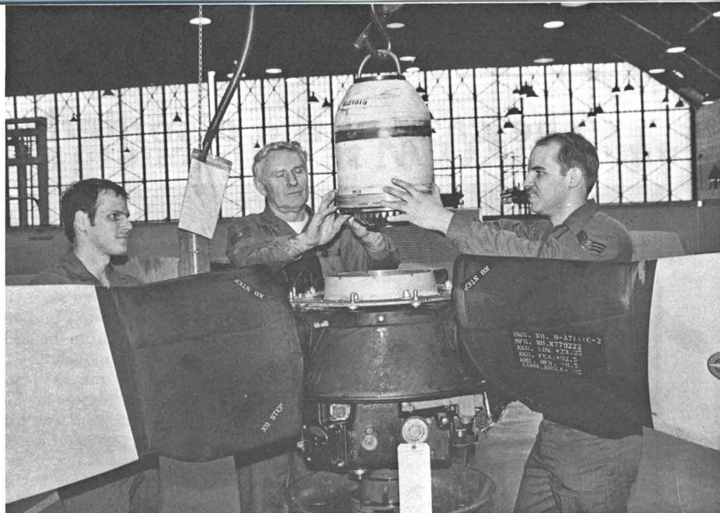
A1C James Whelihan, MSgt. Phil Retelle and Sgt. Michael Hill (left to right) guide the dome assembly for a C-130 propeller onto the propeller housing.
