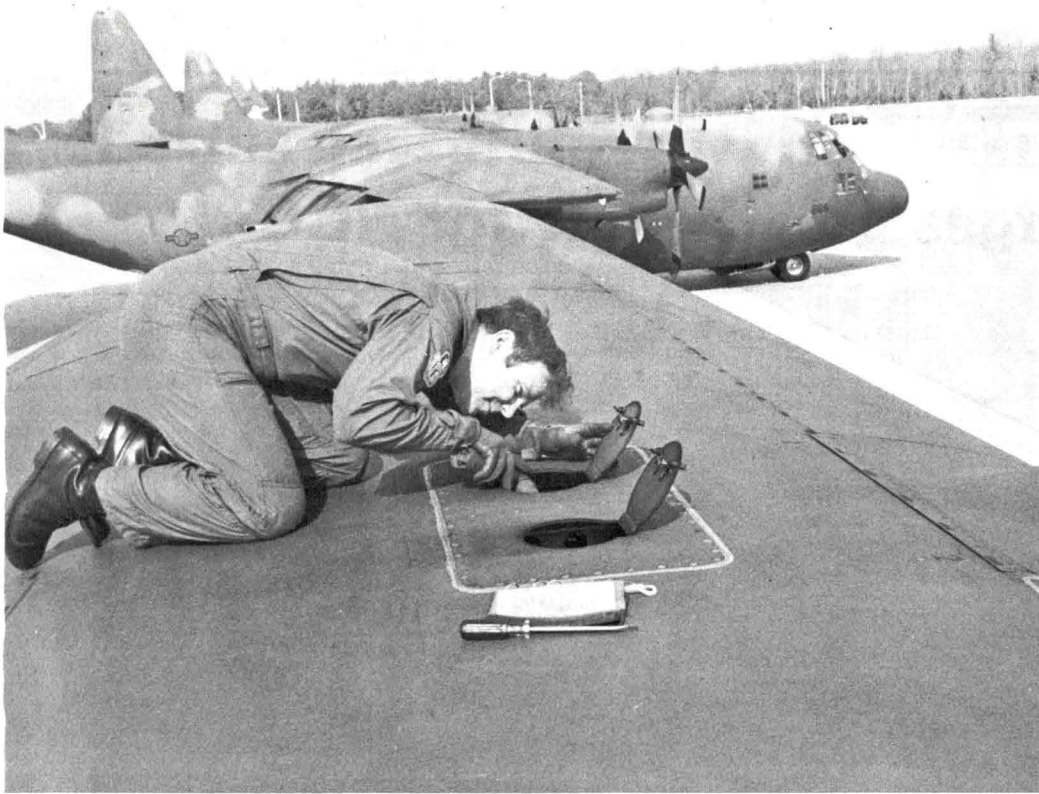
TSgt. Paul Harrison, 337th TAS flight engineer, checks a dry bay in C-130 wing for fuel leaks prior to take off at Pope AFB.
