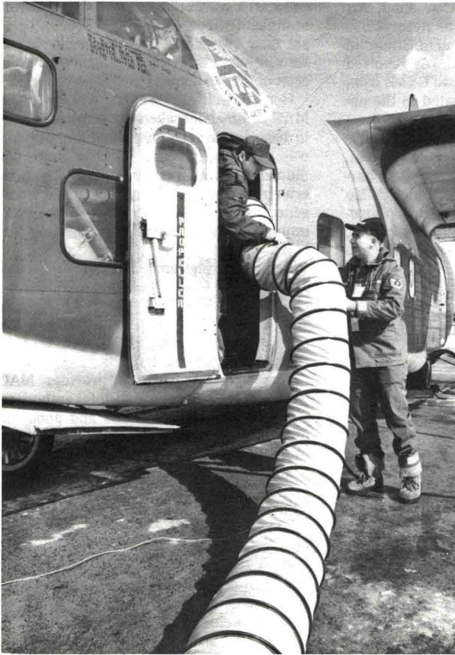
HOT AIR . . . . Maintenance crew member Amn. Steve Boutin, left, and TSgt. Harvey Cook, crew chief, 901 CAMS, place heater hose in a C-123 to provide needed warmth for the electrical equipment.
