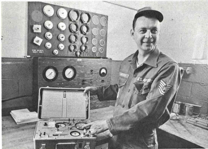
TESTING, TESTING . . . . TSgt. Bernard McCormick, 905 CAMS, demonstrates equipment used to check the oxygen system in an aircraft.
